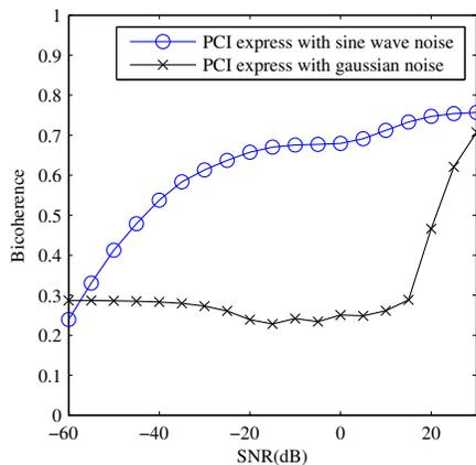
Fig. 7. Peak values in diagonal line average of bicoherence in measured PCI express signal with platform noise
