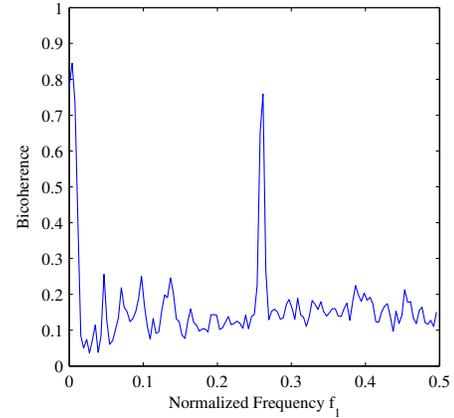
Fig. 5. Diagonal line average of bicoherence in measured PCI express signal
