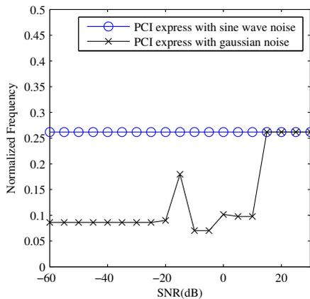
Fig. 6. Peak frequency value in diagonal line average of bicoherence in measured PCI express signal with platform noise
