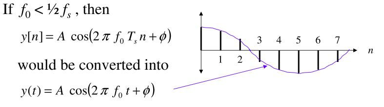
Otherwise, aliasing has occurred, and the converter would reconstruct a cosine wave whose frequency is equal to the aliased positive frequency that is less than  $\frac{1}{2} f_s$
