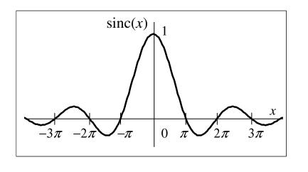
$\operatorname{sinc}(x) = \frac{\sin(x)}{x}$ How to compute sinc(0)? As  $x \to 0$ , numerator and denominator are both going to 0. How to handle it?
